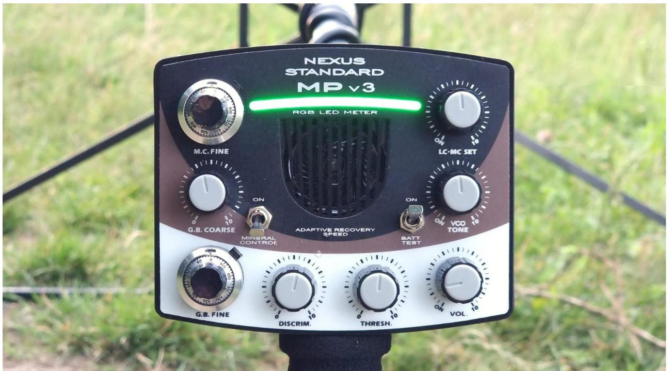
The Nexus Standard MP V3 has eight rotary control knobs and two toggle switches.
